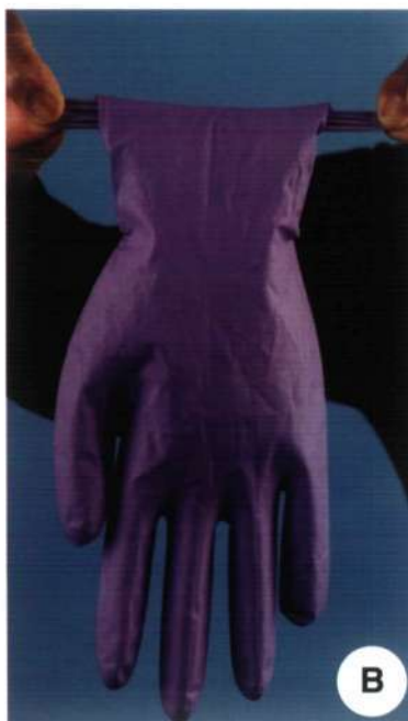
A simple method for detecting fine holes in a glove. A - stretch the cuff of the glove, trapping a small amount of air inside. B - fold the cuff over several times to compress the air. C - if the glove is hole-free, it should remain inflated like this.
